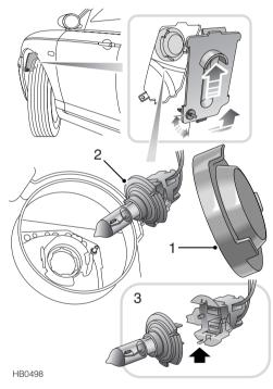
Turn the front wheels to full left or right lock. This provides room to reach into the wheel arch to remove the headlight access panel. Rotate the turnbuckle a quarter turn to left or right to release the access panel (see upper inset). Push the panel up as far as it will go and then disengage the bottom of the panel to remove.
