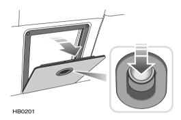
On some models, a fold down hatch is fitted into the rear seat. This enables longer loads to be carried at the same time as one or two rear passengers.
