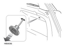
If, for any reason, the fuel filler flap automatic unlocking mechanism fails, the flap can be released manually by pulling a release cord in the loadspace area.
