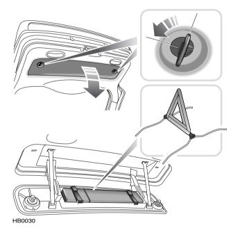
A shallow storage compartment is set into the tailgate trim. This is principally intended to house the emergency warning triangle, available as an accessory from MG Rover dealers.
