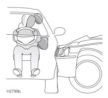
Side airbags are designed to protect the thorax region of the torso and will only deploy in the event of a severe side impact. They will NOT inflate as a result of frontal or rear impacts only.
