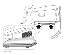
The passenger compartment fuse box is located behind the front passenger glove box.
