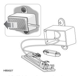
Insert a small flat-bladed screwdriver into the indent on one of the short sides of the lens (see inset in illustration) and carefully prise the lens and bulb carrier from its location. Ease open one of the bulb connectors and pull the bulb to remove.
