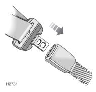
Pull the seat belt steadily over the shoulder and across the chest and, ensuring the webbing is not twisted, insert the metal tongue plate into the buckle nearest the wearer – a 'click' indicates that the belt is securely locked.
