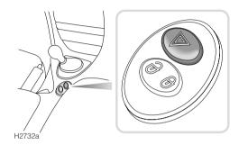
Press to operate. All the direction indicators and direction indicator warning lights will flash together. Use only in an emergency to warn other road users when your car is causing an obstruction or is in a hazardous situation. Remember to switch off before driving away.
