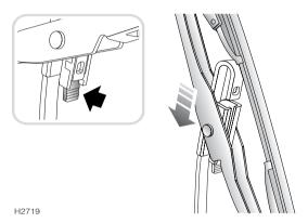
Lift the wiper arm away from the windscreen and set the blade at 90° to the arm as shown. Disconnect the blade by pushing in the locking tab (arrowed in inset), setting the blade at 45° to the arm and sliding the blade down the arm.
