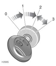
The starter switch is located to the right of the steering column and uses the following sequence of key positions to operate the steering lock, electrical circuits and starter motor:
