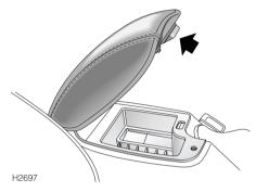
Lift the release catch (arrowed) to open the lid. The cubby box is designed to securely hold tapes or compact discs and the accessory torch available from an MG Rover dealer.
