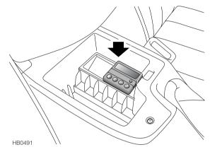
The parking heater timer unit is located in the centre console cubby box. Up to three separate preset operating start times can be programmed, each running for a maximum of 30 minutes.
