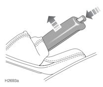
The handbrake operates on the rear wheels only. To apply the handbrake, pull the lever up. Always apply the handbrake FULLY whenever you park the car.
