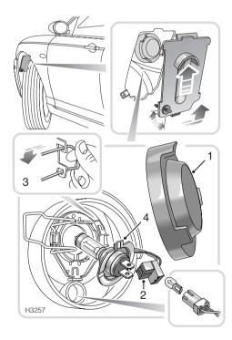
Turn the front wheels to full left or right lock. This will provide room for you to reach into the wheel arch to remove the headlight access panel.
