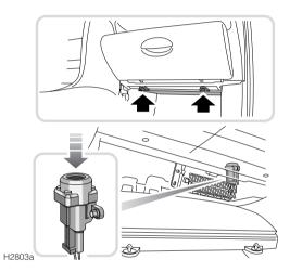
In the event of a collision or sudden impact, an inertia switch automatically cuts off the fuel supply to the engine and, providing the alarm is disarmed, unlocks the doors.
