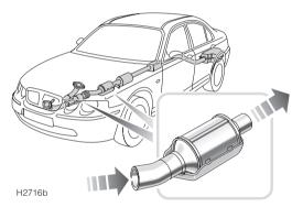
The exhaust system incorporates one or two catalytic converters, which convert poisonous exhaust emissions from the engine into environmentally less harmful gases.
