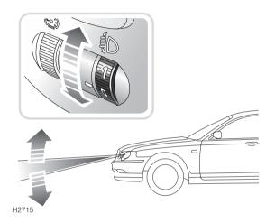
Using the following load conditions as a guide, adjust the headlights by rotating the adjuster wheel (see inset):
