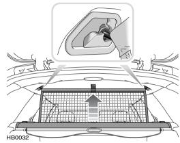
On some cars, the loadspace cover cassette also incorporates a safety net, designed to prevent loose loads and items of luggage from encroaching into the passenger compartment in the event of an accident or emergency manoeuvre.
