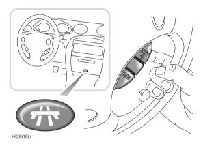
Cruise control enables the driver to maintain a constant road speed without using the accelerator pedal. This is particularly useful for motorway cruising, or for any journey where a constant speed can be maintained for a lengthy period.
