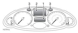
The standard instrument panel features two main clusters of warning lights, one situated in the centre of the pack (1) and the other located at the upper centre of the instrument pack (2).
