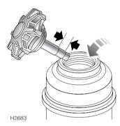
Wipe the filler cap clean to prevent dirt from entering the reservoir. Remove the filler cap and, using a clean lint-free cloth, wipe the dipstick clean. Refit the cap fully and remove again to check the fluid level. If necessary, top-up with a fluid meeting Dexron III specification until the level is between the upper and lower marks on the dipstick (see illustration). DO NOT OVERFILL!
