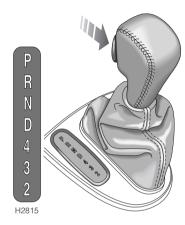
The automatic transmission features a five speed gearbox with three manually selectable modes: Normal (economy), Sport and Snow mode.
