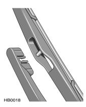
Lift the wiper arm away from the rear screen. The blade is a press fit onto the arm: Grasping the arm firmly with one hand, ease the blade away from the arm.
