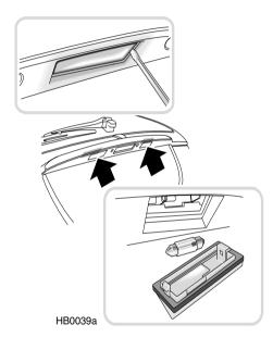
To access a bulb, use a small flat-bladed screwdriver to ease the lens from the underside of the applique (see upper inset - the lever action of the screwdriver will compress the spring retaining clip and enable the lens to be pulled free). Prise the connectors apart to remove the bulb.
