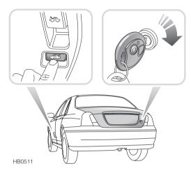
To open, turn the key clockwise in the lock or, from inside the car, press the release button in the driver's footwell. The luggage compartment and interior lights switch on automatically when the boot lid is opened.
