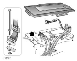
Before disconnecting or removing the battery, disarm the alarm, and ensure that the starter switch and all electrical equipment is turned off.
