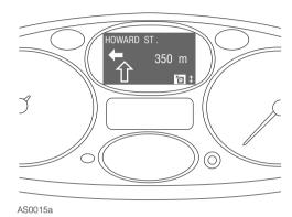
The navigation system shares the larger display panel at the top of the instrument pack with the message centre. From time to time it may be necessary for message centre information to be displayed while the navigation system is in use. In this case, the message centre display will alternate with the navigation display. However, audible information accompanying navigation displays will be unaffected.
