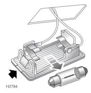
Insert a small flat-bladed screwdriver (preferably with a short handle, due to limited access) into the indent on the left hand side of the light unit, and carefully prise the unit from the glovebox panel. Remove the bulb from its clips.
