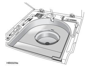
Raise the hinged portion of the loadspace floor (see 'SPARE WHEEL & TOOLS (Tourer)\*', page 224) to reveal the shallow underfloor storage tray. A deeper, circular storage compartment is set into the centre of the tray.
