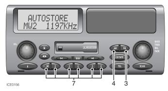
Auto-store enables you to rapidly tune and store the strongest FM and MW radio signals in a single operation. This facility is particularly useful if you are in an unfamiliar area and have little knowledge of local transmitter frequencies.
