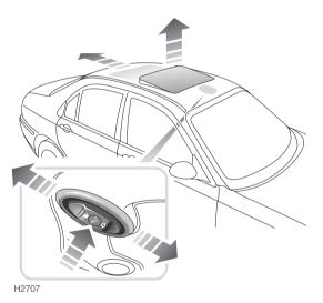
The sunroof can be operated when the starter switch is in the first or second position and for up to 40 seconds after the starter switch is turned off (provided the driver's door is not opened in the meantime).
