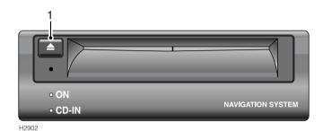
The navigation computer is located on the right hand side of the luggage compartment. Check that the 'ON' indicator light is illuminated, if not, press the eject button (1) to activate the system. Partially insert the navigation CD until it is automatically drawn into the computer (the 'CD-IN' indicator light will illuminate).
