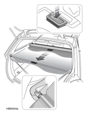
The loadspace cover is a spring-loaded roller blind, which can be pulled from its cassette and secured to hooks at the rear of the loadspace (see lower inset).
