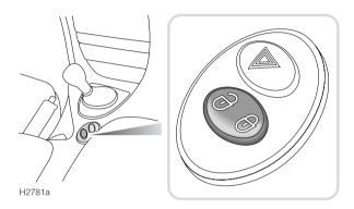
This is a personal security feature which allows the driver to lock (or unlock) all the doors from inside the car (while driving or with the car stationary). Press the closed padlock symbol on the switch to lock (the alarm will not be armed), and the open padlock symbol to unlock.
