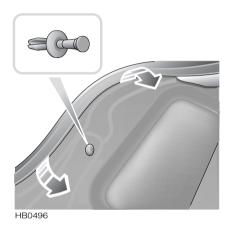
*To remove the fixing:* Use pliers or the flat blade of a screwdriver to lever the head of the fixing away from the boot lining. The fixing can then be pulled from its mounting position.
