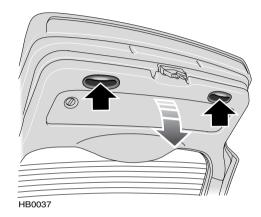
When closing the tailgate, use the two hand grips set into the trim panel on the inside of the tailgate (arrowed in illustration) to pull the tailgate down. When the tailgate is partially closed, release the hand grips and apply light downward pressure on the outside of the tailgate below the number plate to close.
