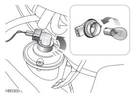
Detach the electrical connector from the rear of the bulb holder by squeezing the clips on both sides of the connector and pulling the connector away from the light unit.
