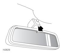
The interior mirror is equipped with a light sensor (arrowed) which activates the automatic dipping function.
