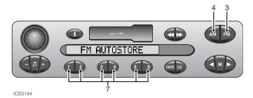
Auto-store enables you to rapidly tune and store the strongest FM and MW radio signals in a single operation. This facility is particularly useful if you are in an unfamiliar area and have little knowledge of local transmitter frequencies.
