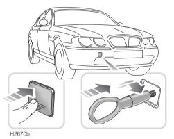
Your car is equipped with a fixed towing point at the rear and a removable towing eye at the front. The front towing eye is stored in the tool kit beneath the loadspace floor when not in use.
