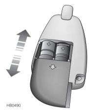
With the back of the remote handset facing uppermost, slide off the battery compartment cover and remove the discharged batteries. Replace with two MN21 12V alkaline batteries, ensuring that the correct battery polarity is maintained.
