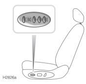
Your car can memorise three different driver seating positions. To store the positions in the system memory, the starter switch must be turned to the first or second position.
