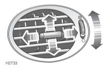
Rotate the thumbwheel down to close or up to open the vents. Direct the air flow by moving the control in the centre of the louvres up or down, or from side to side.
