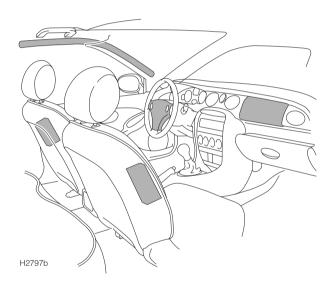
The airbag SRS incorporates front and side airbags for both the driver and front seat passenger.
