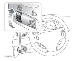
Rotate the control up to increase and down to decrease instrument illumination. The instrument dimmer also controls the illumination of switches, audio system, message centre, trip computer and the satellite navigation system\*.
