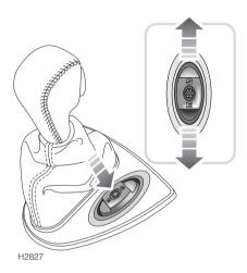
The automatic gearbox has three driver-selectable operating modes: Normal (economy), Sport and Snow. When the starter switch is turned on, the transmission automatically selects the Normal (economy) mode.
