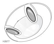
The rear courtesy lights illuminate and extinguish automatically in conjunction with the front courtesy lights. Press the appropriate switch to illuminate the relevant map reading light – press again to switch off.
