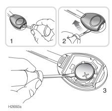
The handset battery should last for approximately three years dependent upon use. It is recommended that you fit an MG Rover YWK10003 or a Panasonic CR2032 replacement battery.
