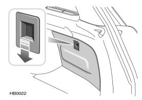
Some cars are equipped with enclosed storage compartments, one on each side of the loadspace. To remove a storage compartment cover, pull the catch down (see inset). When replacing, ensure the catch is pushed up fully to secure the cover in position.
