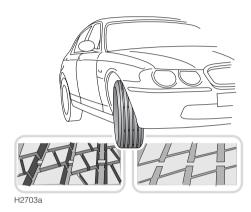
Tyres fitted as original equipment have wear indicators moulded into the tread pattern at several points around the circumference. When the tread has worn down to 1.6 mm, the indicators will come to the surface of the tread pattern, producing the effect of a continuous band of rubber across the width of the tyre.
