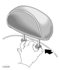
Raise or lower the restraint until the cushion is level with the back of the head.
