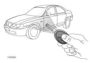
While it is not necessary to point the handset at the car, the handset must be within range when the buttons are pressed. Note that the operating range may vary depending upon handset battery condition and may sometimes be limited by physical and geographical factors beyond your control. From a security point of view, it may not be wise to unlock unless you are close enough to visually confirm that the doors have locked.
