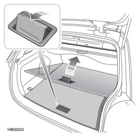
Raise the recessed handle set into the rear of the loadspace floor and raise the floor.
