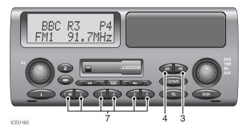
The six pre-set buttons (7) can be used to manually store up to twelve FM stations (six each on FM1 and FM2), twelve MW stations (six each on MW1 and MW2), and six LW stations.
