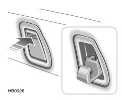
On some cars, two retractable carrying hooks are set into the side trim panels in the loadspace. Use these to secure bags or loose items, which might, otherwise, move around the loadspace in response to the car's momentum.
