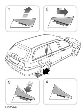
On Tourer models, to ensure adequate stability, even on level ground, it is essential to chock one of the road wheels before raising the car from the ground.
