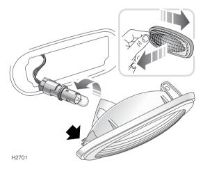
Push the lens firmly towards the front of the car to release the light unit, then withdraw the light from the wing.
