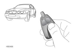
The remote handset supplied with your parking heater, has an approximate unobstructed range of 300 metres, but this range can be substantially reduced by buildings, obstructions or mountainous terrain.
