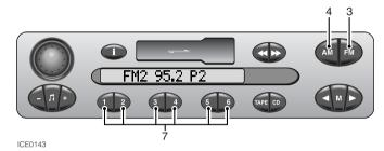
The six pre-set buttons (7) can be used to manually store up to twelve FM stations (six each on FM1 and FM2), twelve MW stations (six each on MW1 and MW2), and six LW stations.
