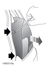
With the tailgate open, use the flat-bladed end of the screwdriver (supplied in the tool kit) to prise open the two flaps on the inboard side of the light unit (where indicated in illustration), to reveal two retaining screws.
