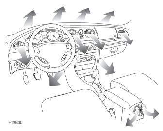
The heating and ventilation system provides fresh or heated air to the interior of the car from the air intake grille in front of the windscreen. Always keep the air intake grille clear of obstructions such as leaves, snow or ice.
