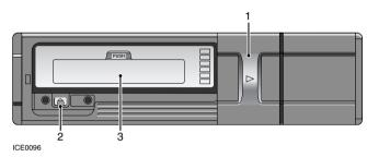
Fully open the sliding cover (1) to insert or remove the magazine. Keep the cover closed at all other times to prevent dust and dirt from entering. Press the button (2) to eject the magazine.
