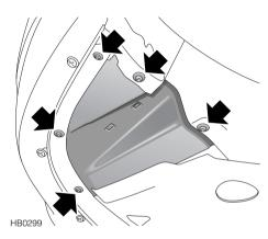
To access the light unit, the small panel immediately below the relevant light must be removed from the underside of the car. This is held in place by five Philips type screws, which must be removed before the panel can be released (see illustration for location of the five screws).
