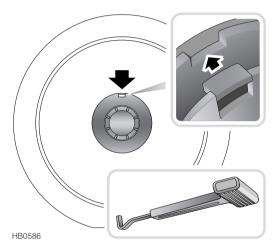
Insert the hooked end of the removal tool into the small rectangular aperture in the wheel bolt cover (arrowed in illustration). Pull the cover from the wheel to gain access to the wheel bolts.
