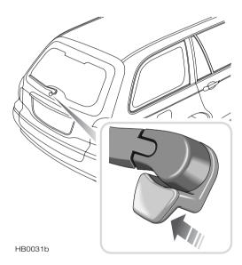
The tailgate window should only be opened when the tailgate is closed. With the central door locking system unlocked (handset unlock button pressed twice, or door key turned to the unlock position twice), operate the switch concealed beneath the rear wiper mounting to open (see illustration).
