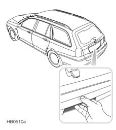
The tailgate and tailgate window are included in the car's central locking system and lock/unlock automatically in tandem with the doors.
