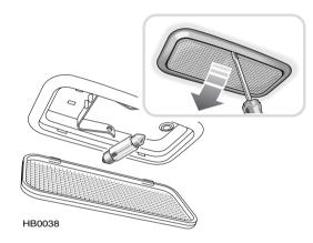
Insert a small flat-bladed screwdriver into the indent on the rear edge of the lens (see inset) and carefully prise the lens from the light unit. Gently spread the flexible contacts to release the bulb.
