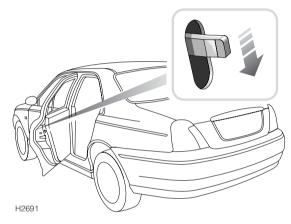
Move the locking levers on the rear doors down to engage the child locks.
