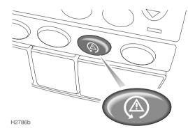
Traction control is entirely automatic in operation. However, the system can be manually overridden by pressing the traction control disable switch (see illustration). The system will then remain disabled until the switch is pressed a second time, or until the starter switch is turned off.
