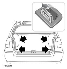
Luggage carried in the loadspace will shift position in the event of an accident or sudden stop. Four lashing rings are set into recesses in the loadspace floor and wheel arches, where shown. Raise the rings from the floor (see inset) and secure all loads before driving.
