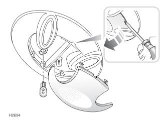
Insert a small flat-bladed screwdriver into the indent at the rear of the lens (see inset) and gently prise the lens from the light unit. Pull the bulbs from their mountings to remove.
