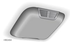
Interior space protection (ultrasonics) is designed to protect the interior of the car from intrusion (entry by a thief through a smashed window, for example). Ultrasonic sensors, mounted on the roof lining, monitor the interior space and activate the alarm if air movement is detected in the passenger compartment.
