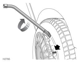
Slide the flat, wedge, end of the wheel wrench behind the edge of the wheel trim (see illustration). Then, working carefully around the wheel, apply a twisting action to the tool to prise the trim from the wheel.
