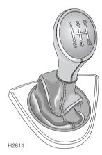
The gear positions are indicated on the gear lever knob.
