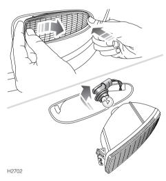
Using hand pressure, push the bottom of the outboard corner of the lens very firmly towards the REAR of the car; at the same time, push the inboard side of the lens firmly towards the SIDE of the car. This will disengage the securing spring and enable the light unit to be pulled from the front of the bumper.
