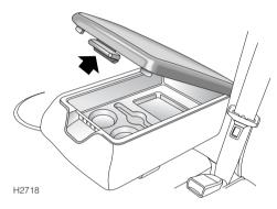
Lift catch (arrowed) to open. Stowage spaces are provided for a pen, memo pad and cup rests for use when the car is stationary. Space is also provided for the optional first aid kit.
