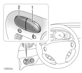
**NOTE:** Both the rear and front fog lights are switched off automatically when the main lighting switch or the starter switch are turned off, and will need to be reselected when the starter switch is turned back on.
