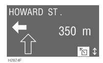
After the chosen route method is selected, the navigation computer displays the distance to the next relevant junction and the direction which should be taken at that junction (a solid arrow).
