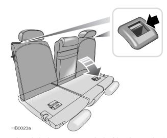
To release the backrest, press one or both of the release catches (as required) shown in the illustration.
