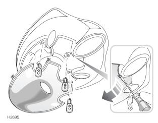
Insert a small flat-bladed screwdriver into the indent at the rear of the lens (see inset) and gently prise the lens from the light unit. Pull the bulbs from their mountings to remove.
