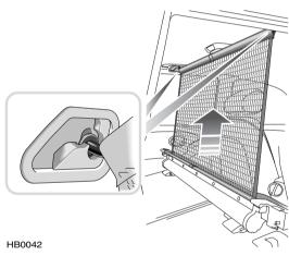
**6.** Pull the central tab towards the roof and hook both sides of the net into the slots set into the roof lining above the cassette (these are integral with the rear seat passenger grab handles).
