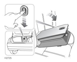
A fold down hatch is fitted in the middle of the rear seat. This enables longer loads to be carried at the same time as two rear passengers.
