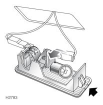
Insert a small flat-bladed screwdriver into the indent on one of the narrow sides of the lens (see arrow in illustration) and carefully prise the unit from its location. Push and twist the bulb to remove.
