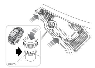
Remove the detachable mesh panel on the driver's side of the car to access the brake fluid reservoir. The fluid level can be seen through the reservoir neck and should be maintained as close to the 'MAX' mark as possible. DO NOT allow the level to drop below the 'MIN' mark.
