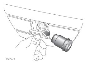
With the starter switch turned on, press the cigar lighter cover to open. Press the lighter in to heat up; when it has reached the correct temperature, it will partially eject and can then be withdrawn for use.
