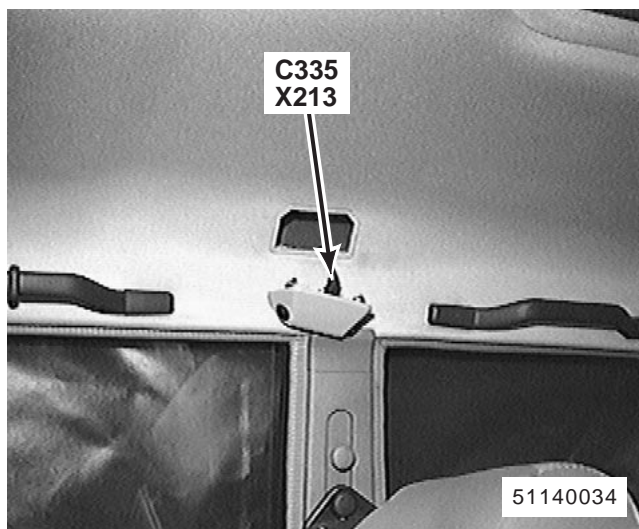
241. top of LH B-post X213 Alarm Sensor C335 (4-B)
