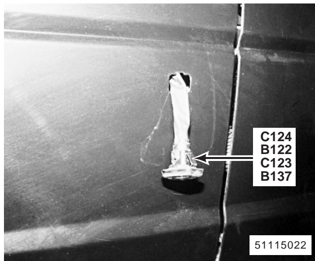
26. LH front side of vehicle (RH similar) B122 Left Repeater Lamp B137 Right Repeater Lamp C123 (2-B) (Right) C124 (2-B) (Left)
