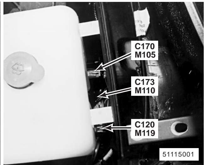
2. LH rear corner of engine compartment M105 Front Screen Wash Pump M110 Headlamp Wash Pump M119 Rear Screen Wash Pump C120 (2-W) C170 (2-R) C173 (2-B)
