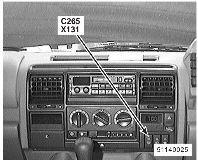
238. centre of fascia X131 Heated Front Screen Switch C265 (5-B)
